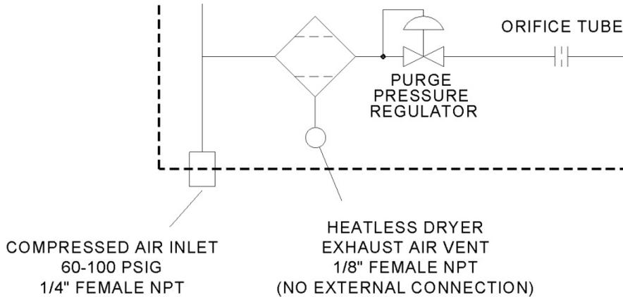
It is located in the lower part of the enclosure and provides dry purge air to the Nafion® membrane sample gas dryer. The heatless dryer operates on the pressure swing adsorption principle where one cylinder acts to dry the air under
