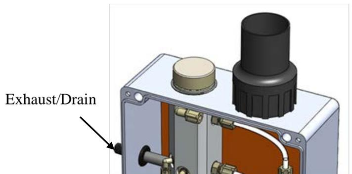
*Connect the line from the eductor outlet to designated collection/exhaust basin containing acid absorption media to prevent release of exhaust to the surrounding area.*
