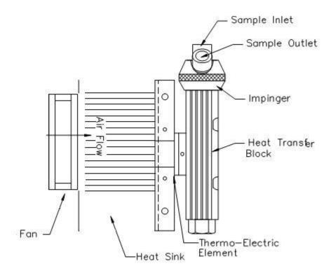
Heat Exchanger, Impinger and Heat Sink Assembly
