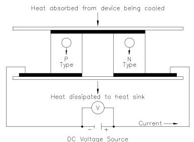
Figure 1: Thermo-electric element (Peltier)
