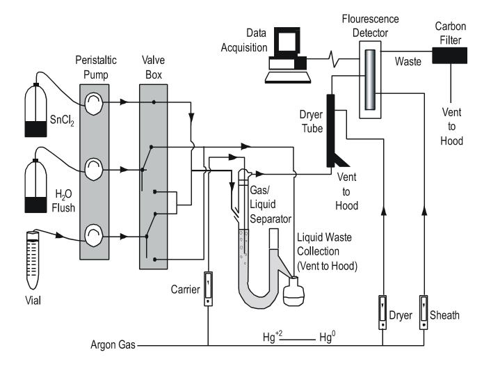
Figure 1: Automated Mercury Fluorescence System
